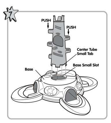
Align the smallest tab on the center tube with the smallest slot in the base. Push down on the track support to "snap" the center tube into place.
